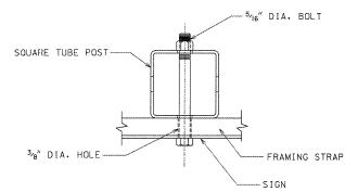
OPTION #2 - FRAMING STRAP WITH MOUNTING HOLE (ALL FRAMING STRAPS SHALL BE 2"  $\times$   $^{1}$  $_{2}$ "  $\times$  REQUIRED LENGTH)
