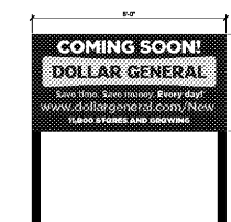
THIS SIGN IS TO BE PROVIDED AND INSTALLED BY THE DEVELOPER OR CONTRACTOR AT THE BEGINNING OF CONSTRUCTION PROJECT.
