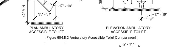
Figure 604.8.2 Ambulatory Accessible Toilet Compartment
