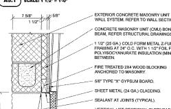
EXTERIOR CONCRETE MASONRY UNIT (CMI) VALL SYSTEM REFER TO WALL SECTIONS CONCRETE MASONRY LINIT (CML), BOND
