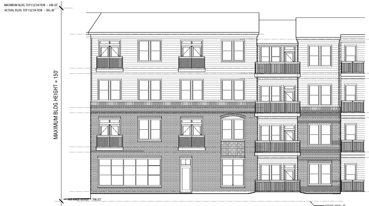
4 CHARLES DRIVE - RIGHT WING ELEV. (POOL) THIS ELEVATION DOES NOT FACE A PUBLIC ROAD AND IS REQUIRED TO HAVE 50% MASONRY. 1/8"=1'-0" TOTAL WALL AREA = 2909 SF TOTAL BRICK AREA = 1862 SF 815 / 1509 = 64% MASONRY
