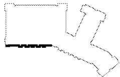
1 CHARLES DRIVE - LEFT WING ELEVATION THIS ELEVATION FACES A PUBLIC ROAD AND IS REQUIRED TO HAVE 80% MASONRY. TOTAL WALL AREA = 6982 SF TOTAL BRICK AREA = 5856 SF 5856 / 6982 = 82.8% MASONRY
