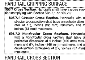
FIGURE 505.7 HANDRAIL CROSS SECTION
