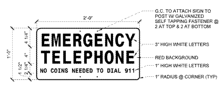
3 SIGNAGE @ TELEPHONE POST 1 1/2' x 1'-0"
