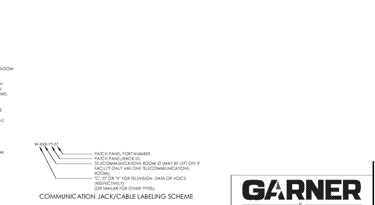
6 COMMUNICATION JACK/CABLE LABELING SCHEME
