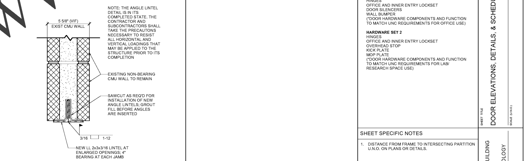
C8 LINTEL DETAIL AT NEW OPENINGS 0 1 2 3 4 6 12 IN
