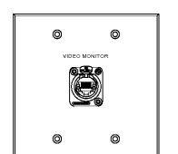
2 VM1.1 THRU 2 VM1.3 VIDEO MONITOR I/O PLATE 2-GANG BACK BOX RECESSED FLUSH ON WALL 84" A.F.F. BACK BOX PROVIDED AND INSTALLED BY E.C. FACEPLATE PROVIDED AND INSTALLED BY P.S.C.
