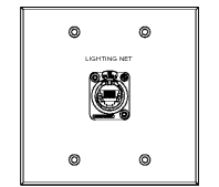
2 LN1.1 THRU 2 LN1.7 LIGHTING NETWORK / DMX PLATE 2-GANG BACK BOX RECESSED FLUSH ON WALL 18" A.F.F. BACK BOX PROVIDED AND INSTALLED BY E.C. FACEPLATE PROVIDED AND INSTALLED BY P.S.C.
