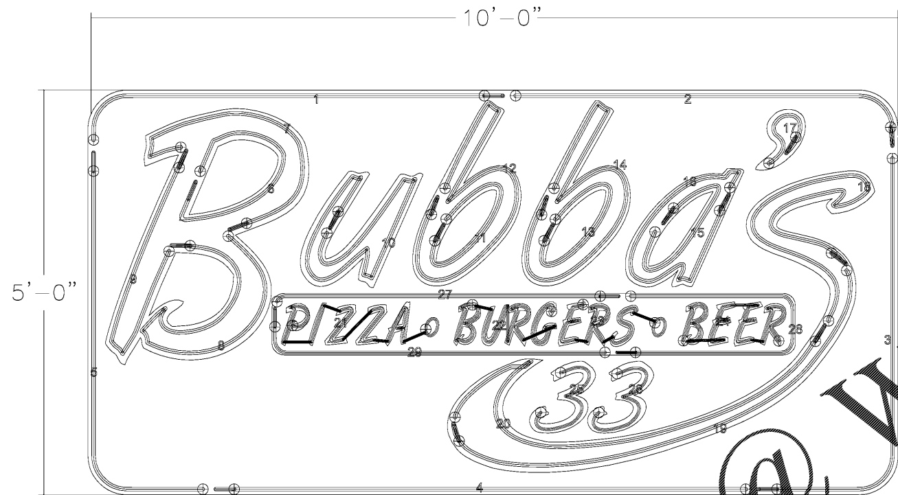
BUBBA'S 5'-0" x 10'-0" CABINET WALL SIGN W/ OFCL
