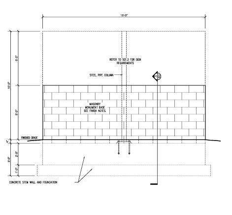
NOTE: VERIFY LOCATION PRIOR TO POURING TO ASSURE NO INTERFERENCE WITH UTILITIES
