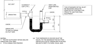
1. ALLOW SUFFICIENT SPACE BELOW DRAIN PAIN FOR TRAP
