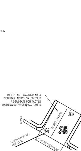
7 Sidewalk Detail SCALE: 1 1/2" = 1'-0"
