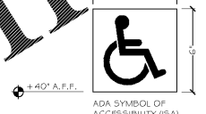
ADA SYMBOL OF ACCESSIBILITY (SA) DECAL TO BE LOCATED ON STOREFRONT GLASS ADJACENT TO ALL ACCESSIBLE DOORS. WINDOW DECAL SCALE: NONE
