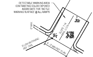
5 Handicap Ramp Detail SCALE: 1/4" = 1'-0"
