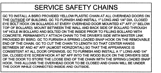
20 SERVICE BAY SAFETY CHAIN F1 SCALE: 1/2"=1'-0"
